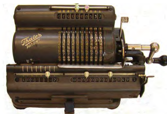
Illustration 12: Multiplicatrice de technologie Odhner
