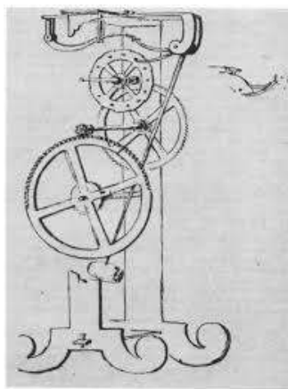
(a) Galileo's pendulum clock drawn by Viviani (Pendulum clock, n.d)
