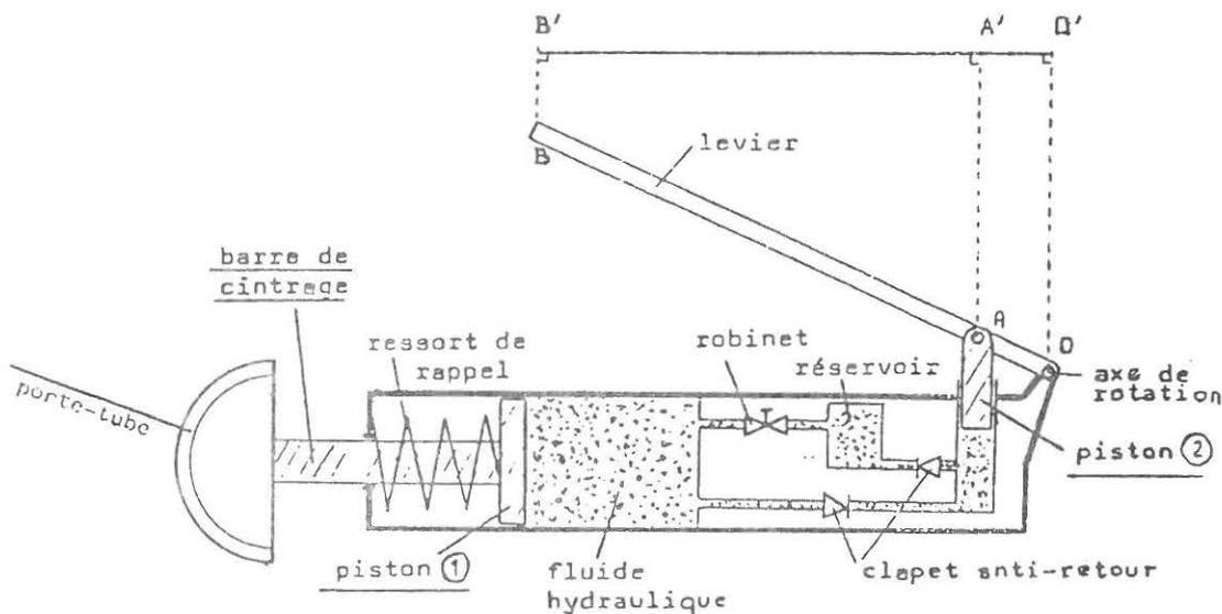
SCHEMA D'UNE CINTREUSE A VERIN HYDRAULIQUE
