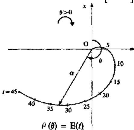
$$\text{avec} \quad E(t) = \left[ r^2 + \frac{t}{a} \right]^{\frac{1}{2}} - r \quad \text{et} \quad a = \frac{\pi}{eV}$$
